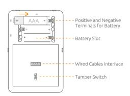
Tamper Switch: The tamper switch will be activated if case is opened.
